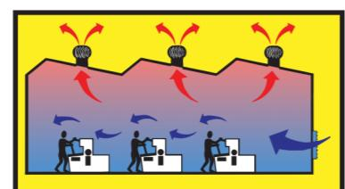
THE WHIRLING TURBINE ACTION REMOVES CONVECTED HEAT AND POLLUTION BUILD-UP
